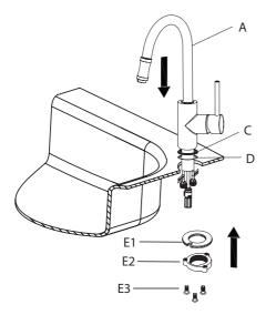
Insert faucet body (A) into hole on deck or sink with base (C) and base o-ring (D) attached. Attach mounting hardware assembly (E)
