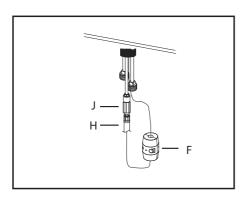
Attach weight (F) to lowest point vertically on spray hose (H)
