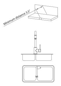
The minimum distance between the faucet hole and the wall should be 3.5"
