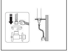
Connect and tighten waterlines (G) to angle stops. Turn on the angle stops and check for leaks
