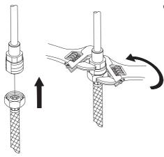
Connect waterlines (G) to hot and cold copper lines on faucet
