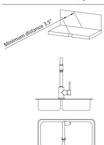
If the distance between the faucet hole and the wall is less than 3.5," position the faucet lever 30° to 90° off the wall to allow for full operation
